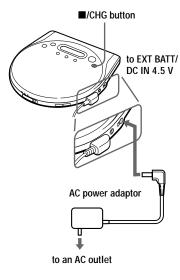
The CD player charges the batteries. The "CHG" indicator turns on in the display, and the indicator sections of [ ] light up in succession. When the batteries are completely charged, the "CHG" and [ ] indicators turn off.
